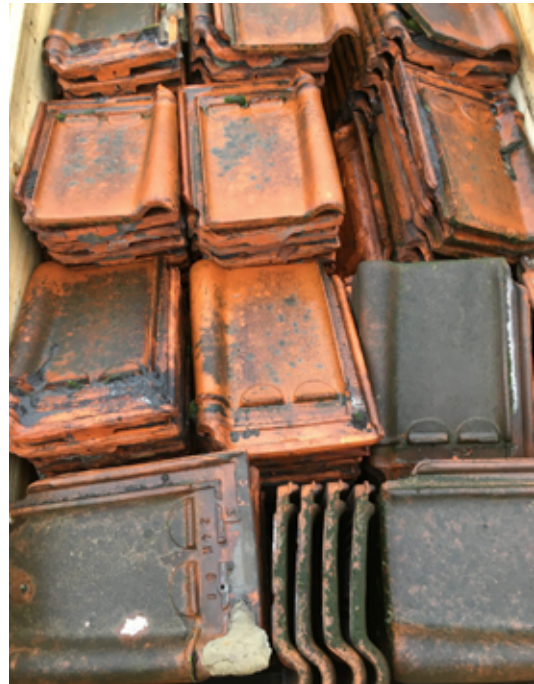
Aesthetic appearance of tiles after removal from roof © Wienerberger®
