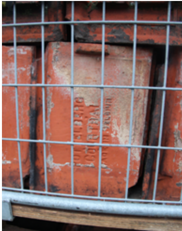
Example of indication of tile provenance on its back (© Buildwise)
