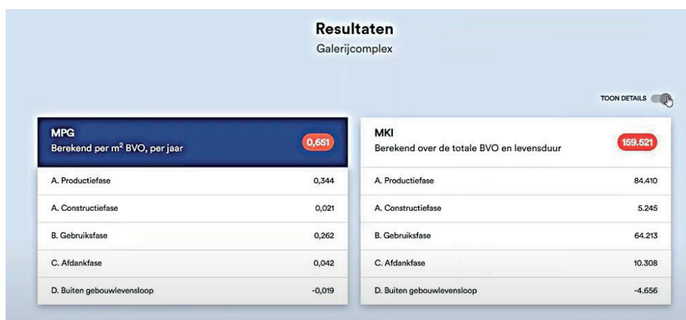
Figure 26: Representation of the results of the MPG calculation per life cycle stage in the GPR Materiaal tool 28 .
