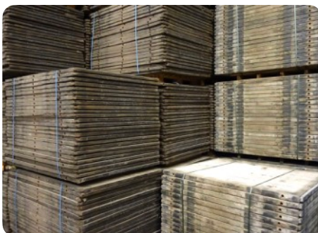
Reclaimed timber formwork steenschotten panels
