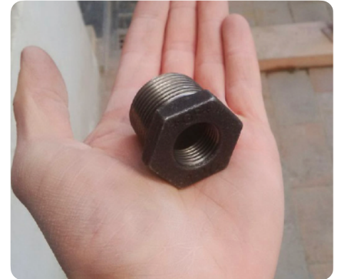
Replacement of outlet plugs © LIONEL BILLIET
