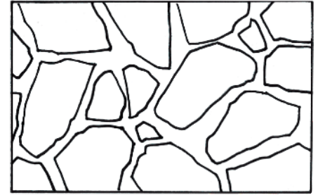
Opus incertum: format allowing to work with any fragments of broken slabs.
