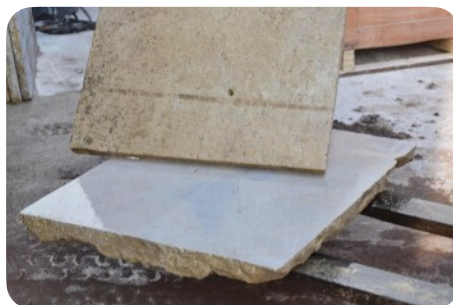
Thickness sawing of the slabs, thicker and irregular bottom part
