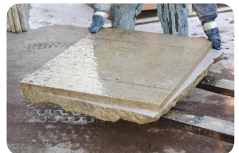
Thickness sawing of the slabs, smooth and even top part
