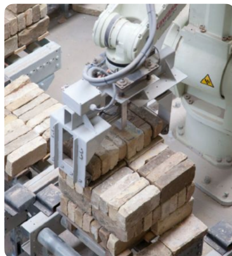
Mechanised sorting and packaging of reclaimed bricks © Gamle Mursten (DK)
