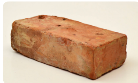
Beerssesteen-type extruded reclaimed brick (BE)
