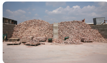
Storage of dismantled bricks before sorting and cleaning, at a professional dealer
