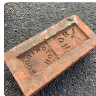
Accrington type mechanically moulded reclaimed brick (UK)
